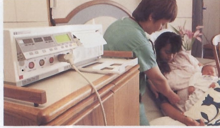
An HP M1350B fetal monitor records Laurie Kealiinohomoku's blood pressure. Vital signs are transmitted to an HP OB Tracevue station.
